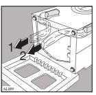
Place the machine in an upright position and remove the three plastic spacers.
